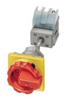
EMERG. STOP SWITCH 3-POLE IU=32, P/AC-23A AT 400V=11.5KW FLOOR MOUNTING DIN RAIL/TWO-HOLE MOUNTING ROTARY ACTUATOR RED/YELLOW (EMERG. STOP)
