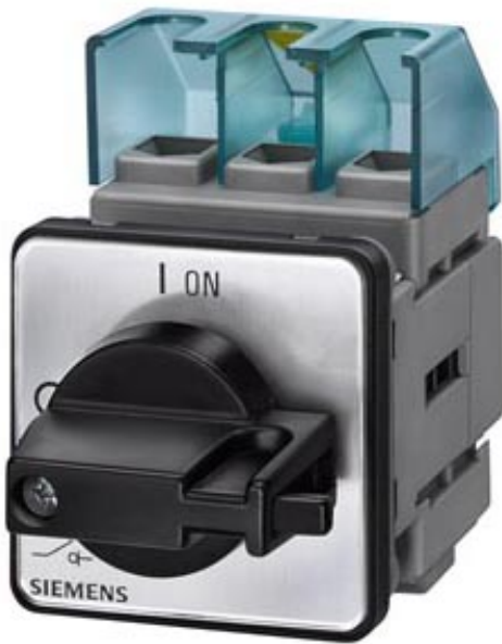
MAIN CONTROL SWITCH 3-POLE IU=25, P/AC-23A AT 400V=9,5KW FRONT MOUNTING CENTRAL- HOLE MOUNTING KNOB BLACK
