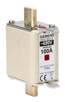
LV HRC FUSE LINK GL/GG WITH NON-INSULATED GRIP LUGS WITH COMBINATION INDICATOR SIZE 00, 100A, AC 690V/DC 250V
