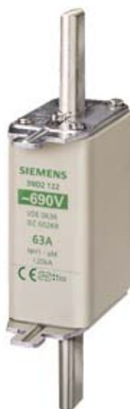
LV HRC FUSE LINK A.M. W. NON-INSULATED GRIPPING LUGS SIZE 1, 100A, AC 690 V
