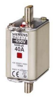
LV HRC FUSE LINK GL/GG WITH NON-INSULATED GRIP LUGS WITH COMBINATION INDICATOR SIZE 00, 40A, AC 690V/DC 250V
