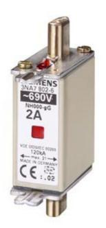
LV HRC FUSE LINK GL/GG WITH NON-INSULATED GRIP LUGS WITH COMBINATION INDICATOR SIZE 000, 32A, AC 690V/DC 250V
