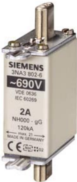
LV HRC FUSE LINK GL/GG WITH NON-INSULATED GRIP LUGS WITH FRONT INDICATOR SIZE 000, 2A, AC 690V/DC 250V
