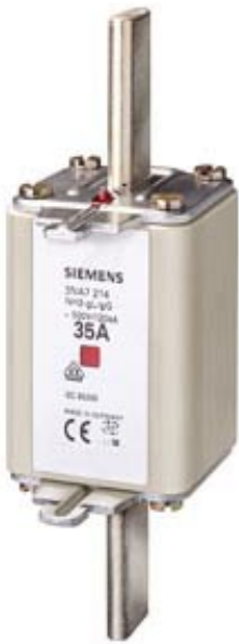
LV HRC FUSE LINK GL/GG WITH NON-INSULATED GRIP LUGS WITH COMBINATION INDICATOR SIZE 2, 35A, AC 500V/DC 440V
