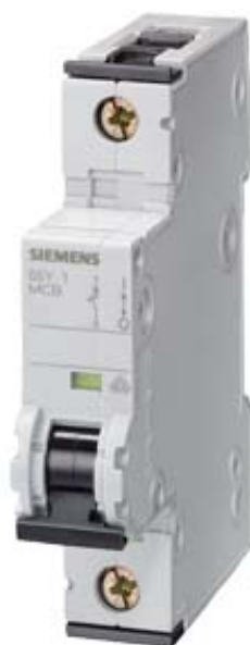
CIRCUIT BREAKER CURR. SENS DC 220V AC 230/400V 10KA, 1-POLE, C, 50A
