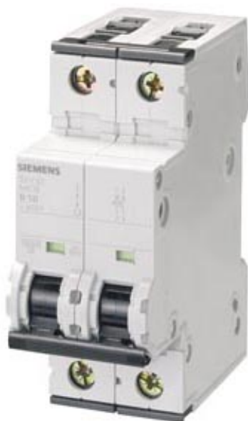
CIRCUIT BREAKER 400V 10KA, 2-POLE, D, 32A, D=70MM
