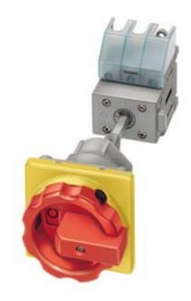
EMERG. STOP SWITCH 4-POLE IU=25, P/AC-23A AT 400V=9.5KW FLOOR MOUNTING DIN RAIL/TWO-HOLE MOUNTING ROTARY ACTUATOR RED/YELLOW (EMERG. STOP)
