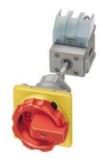
EMERG. STOP SWITCH 4-POLE IU=32, P/AC-23A AT 400V=11.5KW FLOOR MOUNTING DIN RAIL/TWO-HOLE MOUNTING ROTARY ACTUATOR RED/YELLOW (EMERG. STOP)
