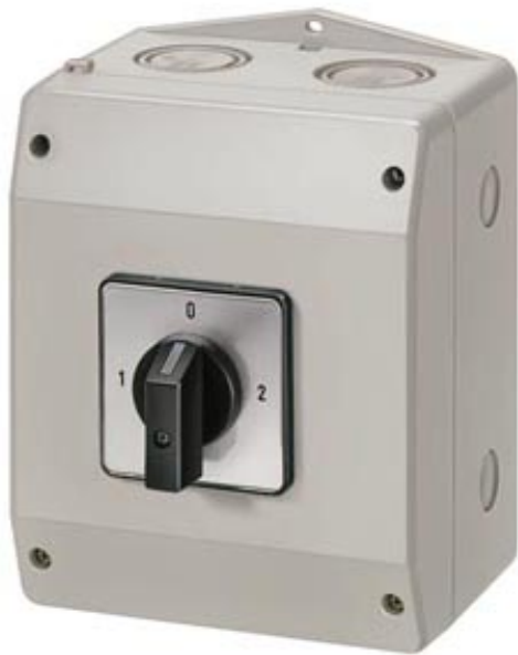
CHANGEOVER SWITCH 3-POLE IU=25, P/AC-23A AT 400V=9,5KW 2 N-TERMINAL MOULDED- PLASTIC ENCLOSURED, IP65
