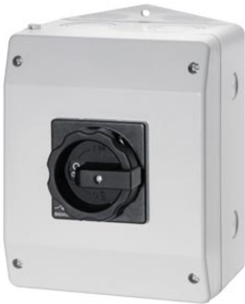
MAIN SWITCH 6-POLE IU=25, P/AC-23A AT 400V=9,5KW 2 N-TERMINAL MOULDED- PLASTIC ENCLOSURED, IP65
