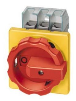
EMERG. STOP SWITCH 4-POLE IU=25, P/AC-23A AT 400V=9.5KW 1NO+1NC, FRONT MOUNTING CENTER HOLE MOUNTING ROTARY ACTUATOR RED/YELLOW (EMERG. STOP)
