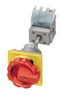
EMERG. STOP SWITCH 4-POLE IU=16, P/AC-23A AT 400V=7.5KW FLOOR MOUNTING DIN RAIL/TWO-HOLE MOUNTING ROTARY ACTUATOR RED/YELLOW (EMERG. STOP) FOUR-HOLE MOUNTING
