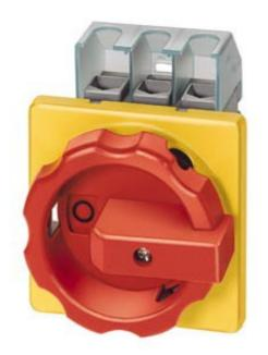
3-P. MAIN CTR. SWITCH IU=16, P/AC-23A AT 400V=7.5KW FRONT MOUNTING 4-HOLE MOUNTING ROTARY ACTUATOR BLACK
