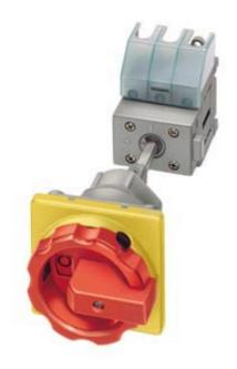
EMERG. STOP SWITCH 3-POLE IU=16, P/AC-23A AT 400V=7.5KW FLOOR MOUNTING DIN RAIL/TWO-HOLE MOUNTING ROTARY ACTUATOR RED/YELLOW (EMERG. STOP) FOUR-HOLE MOUNTING
