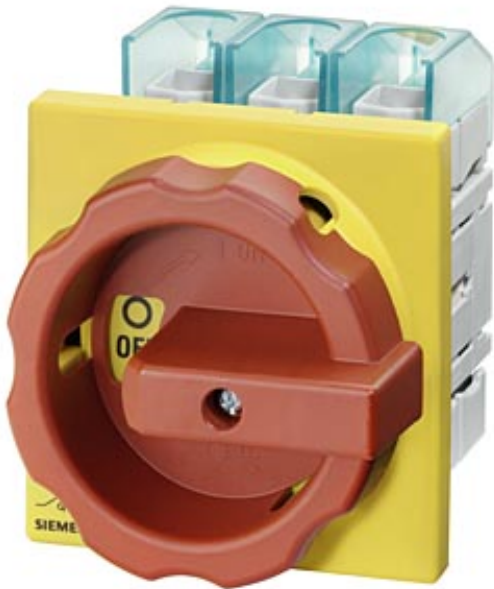
MAIN/EMERG. STOP SWITCH 3-POLE IU=100, P/AC-23A AT 400V=37KW FRONT MOUNTING FOUR-HOLE MOUNTING ROTARY ACTUATOR RED/YELLOW (EMERG. STOP)
