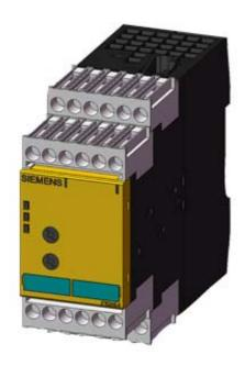
SIRIUS SAFETY RELAY FOR SAFETY-ORIENTED STANDSTILL MONITORING, 24V DC, 45.0MM, SCREW TERMINAL, FK INSTANT.: 3NO 1NC, FK DELAYED: 0, MK: 3, AUTO START, BASIC UNIT, MAX. ACHIEV. CAT. EN954-1: 4, MAX. ACHIEV. SIL TO IEC61508:3,
