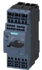
CIRCUIT-BREAKER SZ S0, FOR MOTOR PROTECTION, CLASS 10, A-REL. 7...10A, N-REL. 130A SPRING-L. CONNECTION, STANDARD SW. CAPACITY W. TRANSVERSE AUX. SWITCH 1NO+1NC
