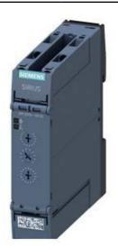
TIME RELAY, MULTI-FUNCTION, 2 CO CONT., 27 FUNCT., 15 TIME SET. RANGES (1, 3, 10, 30, 100) (S/MIN/HR), 400...440 V AC AT AC 50/60HZ, LED, SCREW TERMINAL
