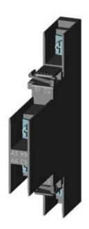
LATERAL AUX.SWITCH BLOCK,SIDE, 1NO+1NC, CURR.PATH: 1NC, 1NO, FOR MOTOR CONTACTORS, SZ S0, RING CABLE LUG CONNECTION R: 31/32, 43/44 L: 51/52, 63/64
