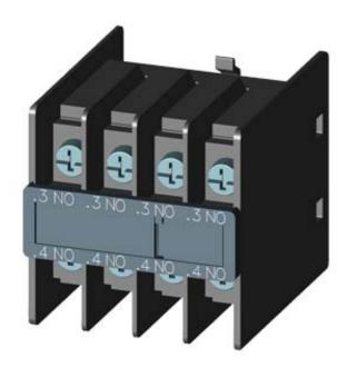
AUX.SWITCH BLOCK,FRONT,4NO, CURR.PATH: 1NO, 1NO, 1NO, 1NO, F. CONT. RELAYS A. MOTOR CONT., SZ S00 AND S0, RING CABLE LUG CONNECTION .3 / .4,.3 / .4,.3 / .4
