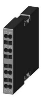
LATERAL AUX.SWITCH BLOCK,SIDE, 2NO, CURR.PATH: 1NO, 1NO, FOR MOTOR CONTACTORS, SZ S00, SPRING-LOADED TERMINAL R: 23/24, 33/34 L :43/44, 53/54
