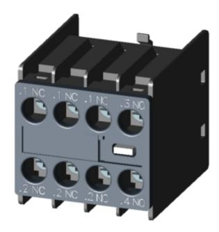
AUX.SWITCH BLOCK,FRONT,1NO+3NC, CURR.PATH: 1NC, 1NC, 1NC, 1NO, F. CONT. RELAYS A. MOTOR CONT., SZ S00 AND S0, SCREW TERMINAL .1 / .2,.1 / .2,.1 / .2,.3 / .4
