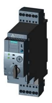
DIRECT STARTER 690 V, 24 V AC/DC, 50 ... 60 HZ, 1 ... 4 A, IP20, CONNECTION MAIN CIRCUIT: SPRING-LOADED TERMINAL, CONNECTION AUXILIARY CIRCUIT: PLUGGABLE, WITHOUT TERMINALS
