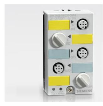
ASISAFE MODULE K45F TWO SAFE INPUTS 2FDI AND TWO STANDARD OUTPUTS 2DO W. AUX. VOLTAGE SUPPLY UAUX 24V DC MOUNTING PLATE 3RK19012EA00 TO BE ORDERED SEPARATELY 2 X STANDARD OUTPUTS 1A, OUTPUT SUPPLY FROM 24 V DC. 4 X M12 SOCKET. MOUNTING PLATE 3RK19012EA00 TO BE ORDERED SEPARATELY.
