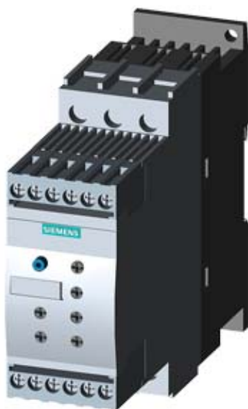
SIRIUS SOFT STARTER, S0, 25A, 15KW/500V, 40 DEGR., AC 400-600V, AC/DC 24V, SCREW TERMINALS
