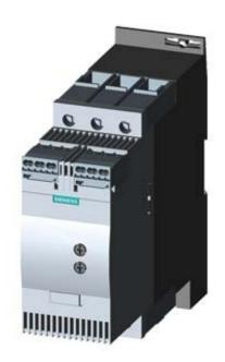
SIRIUS SOFT STARTER, SIZE S2, 45A, 22KW/400V, 40 DEGREES, 200-480V AC, 110-230V AC/DC, SPRING-LOADED TERMINALS
