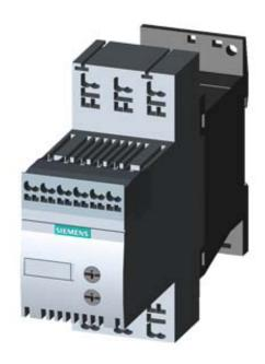
SIRIUS SOFT STARTER, SIZE S00, 9A, 4KW/400V, 40 DEGREES, 200-480V AC, 110-230V AC/DC, SPRING-LOADED TERMINALS
