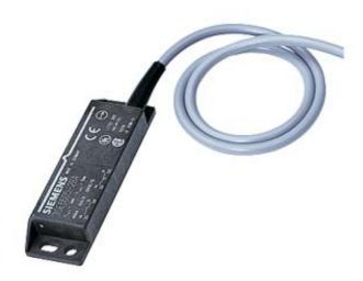
MAGNETIC SWITCH SWITCH BLOCK, RECTANGULAR LARGE 25X88 MM, CONTACTS 1NC/1NO, WITH M8 PLUG 4-POLE, PIN ASSIGN.: PIN1=21, PIN2=22, PIN3=13, PIN4=14
