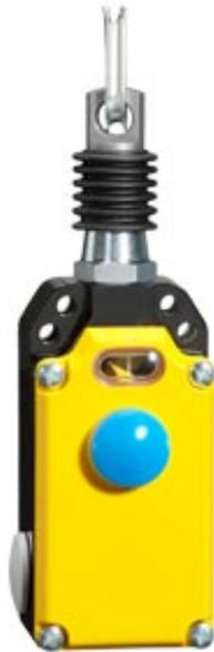
SIRIUS CABLE-OPER. SWITCH METAL HOUSING,2X M20X1.5 2NC, LATCHES ACC. EN ISO 13850 BUTTON RESET FOR CABLES UP TO TO 10M
