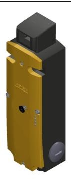
SAFETY POSITION SWITCHES WITH SOLENOID INTERLOCKING LOCKING FORCE 2600N, 5 DIR. OF APPROACH METAL ENCLOSURE, M12 CONNECTOR, ASISAFE INTEGRATED CH1=ACTUATOR 1NC, CH2=MAGNET 1NC SPRING-ACTUATED LOCK, AUX. RELEASE ON FRONT MAGNET VOLTAGE 24V
