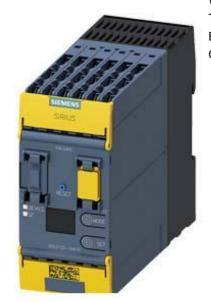
SIRIUS SAFETY RELAY BASIC UNIT 3SK2 SERIES 20 F-DI, 4 F-DQ, 2 DQ, 24 V DC PARAMETERIZABLE VIA SIRIUS SAFETY ES WIDTH 45MM SCREW TERMINALS UP TO SIL3 (IEC 61508) UP TO PERFORMANCE LEVEL E (ISO 13849-1) 3SK1 OUTPUT EXPANSIONS AND 3RM1 FAIL-SAFE MOTOR STARTER CONNECTABLE VIA DEVICE CONNECTOR
