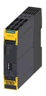
SIRIUS SAFETY RELAY BASIC UNIT ADVANCED SERIES RELAY ENABLING CIRCUITS 3 NO CONTACTS + RELAY SIGNALING CIRCUIT 1 NC CONTACT US = 24 V DC SCREW TERMINAL
