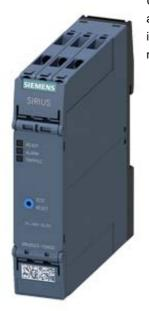
Thermistor motor protection relay Device for warning and switching-off 22.5 mm enclosure screw terminal 1 NO contact + 1 CO contact US = 24 V-240 V AC/DC Manual/Auto/Remote reset with ATEX approval 3 LEDs (READY/WARNING/TRIPPED) Safe galvanic isolation Test/reset button Wire break monitoring Short circuit monitoring non-volatile 2 separate PTC sensor circuits
