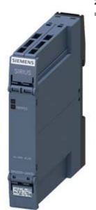
Thermistor motor protection relay Compact evaluation unit, 17.5 mm enclosure, spring-type terminals, 1 changeover contact, US = 24 V-240 V AC/DC, Auto RESET, suitable for bimetallic switch, supply =output voltage, 1 LED (tripped)
