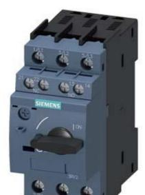
CIRCUIT-BREAKER SZ S0, FOR MOTOR PROTECTION, CLASS 10, A-REL. 3.5...5A, N-REL. 65A SCREW CONNECTION, STANDARD SW. CAPACITY W. TRANSVERSE AUX. SWITCH 1NO+1NC
