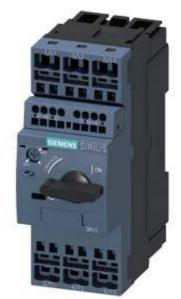
CIRCUIT-BREAKER SZ S0, FOR MOTOR PROTECTION, CLASS 10, A-REL. 5.5...8A, N-REL. 104A SPRING-L. CONNECTION, STANDARD SW. CAPACITY W. TRANSVERSE AUX. SWITCH 1NO+1NC
