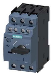
CIRCUIT-BREAKER SZ S0, FOR MOTOR PROTECTION, CLASS 10, A-REL. 2.8...4A, N-REL. 52A SCREW CONNECTION, STANDARD SW. CAPACITY W. TRANSVERSE AUX. SWITCH 1NO+1NC
