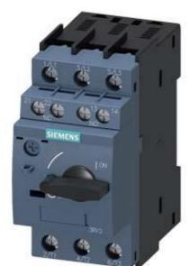
CIRCUIT-BREAKER SZ S0, FOR MOTOR PROTECTION, CLASS 10, A-REL. 4.5...6.3A, N-REL. 82A SCREW CONNECTION, STANDARD SW. CAPACITY W. TRANSVERSE AUX. SWITCH 1NO+1NC
