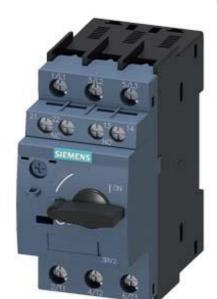
CIRCUIT-BREAKER SZ S0, FOR MOTOR PROTECTION, CLASS 10, A-REL. 5.5...8A, N-REL. 104A SCREW CONNECTION, STANDARD SW. CAPACITY W. TRANSVERSE AUX. SWITCH 1NO+1NC
