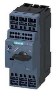
CIRCUIT-BREAKER SZ S0, FOR MOTOR PROTECTION, CLASS 10, A-REL.1.8...2.5A, N-REL.33A SPRING-L. CONNECTION, STANDARD SW. CAPACITY W. TRANSVERSE AUX. SWITCH 1NO+1NC
