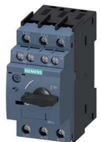
CIRCUIT-BREAKER SZ S0, FOR MOTOR PROTECTION, CLASS 10, A-REL. 1.4...2A, N-RELEASE 26A, SCREW CONNECTION, STANDARD SW. CAPACITY W. TRANSVERSE AUX. SWITCH 1NO+1NC
