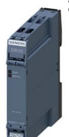
Thermistor motor protection relay Compact evaluation unit 17.5 mm enclosure Screw terminal 1 NO contact, 1 NC contact US = 24 V AC/DC Auto RESET suitable for bimetallic switch 2 LEDs (Ready/Tripped) galvanic isolation
