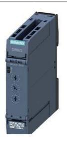
TIME RELAY, MULTI-FUNCTION, 2 CO CONT., 27 FUNCT., 15 TIME SET. RANGES (1, 3, 10, 30, 100) (S/MIN/HR), 400-440V AC AT AC 50/60HZ, LED, SPRING-LOADED TERMINAL (PUSH-IN)
