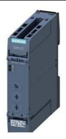
TIME RELAY, MULTI-FUNCTION, 2 CO CONTACTS, 27 FUNCTIONS, 15 TIME SET. RANGES (1,3,10, 30,100) (S/MIN/HR), 24V AC/DC AT AC 50/60HZ, LED, SPRING-LOADED TERMINAL (PUSH-IN)
