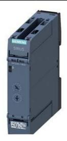
TIMING RELAY, ELECTRONIC, OFF-DELAY, WITHOUT CONTROL SIGNAL OR NON-VOLATILE TIMING RELAY DEFINITE PASSING MAKE CONTACT, 7 TIME SET. RANGES 0.05...600S, 24 V AC/DC, 2 CO CONTACTS, W. LED, SCREW TERMINAL
