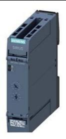
TIME RELAY, ELECTRONIC, WITH STAR-DELTA FUNCTION, 1...20S, TRACK. T.. 30...600S, 3 CONTACTORS, WITH COMMON ROOT, 12...240V AC/DC AT AC 50/60HZ, LED, 0.85 ...1,1US
